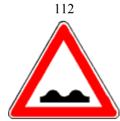
Rough Road. Indicates uneven stretches of road.
