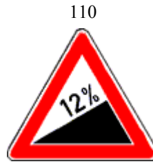
Dangerous Upgrade. Posted before steep upgrades; indicates degree of upgrade.
